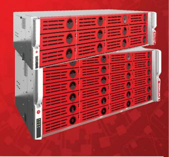
JBOD solutions from Tyrone Opslag FS2 is the perfect combination for expanding your storage needs. We have a series of JBOD to suite all kind of requirements. The hard disk box avaiable in various sizes are suitable for SAS and SATA Hard Drives. It uses the SAS controller to connect to the main box or to other JBOD. Please speak to your local product expert on suitable connectivity and other details or write to <a href="mainto:support@tyronesystems.com">support@tyronesystems.com</a>
